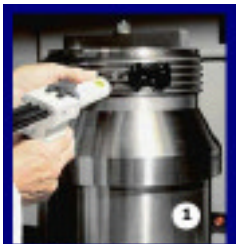
Figure 1: Producing a polymer replica using a hand dispensing gun, a twin pack cartridge and a disposable mixing-nozzle.
