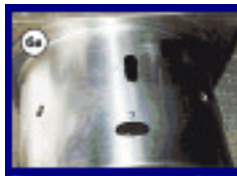
The accurate measurement of the surface finish of a marine main-engine crosshead pin (6a) by in-situ replication and laboratory assessment by interferometry. (Microset 101XP replica measured uncoated and results presented in 3-D interference display mode, Figure 6b).
